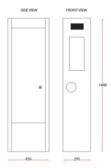
**Struttura** Epoxy powder coated steel, black plexiglass
